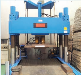
07. Insert Lead-Plug
