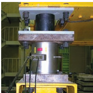
▲ High Damping Rubber Bearing 실험사진
